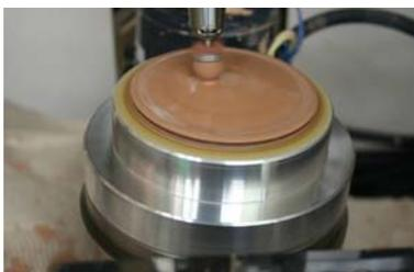
Fig. 6 Polishing machining for aspheric surface
