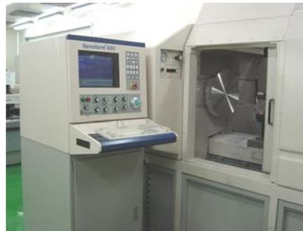
Fig. 1 The system of ultra precision lathe
