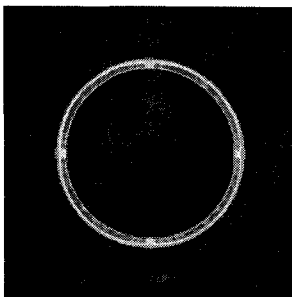
Fig. 5 Equivalent plastic strain for copper ring at 15.64 \mu sec
