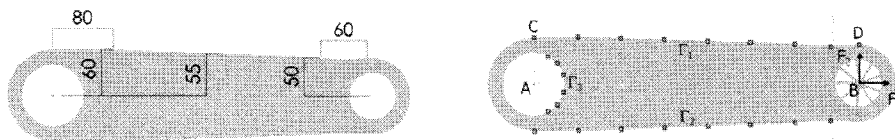
Fig.4. Illustration of Torque arm: Initial design variables and stress check points
