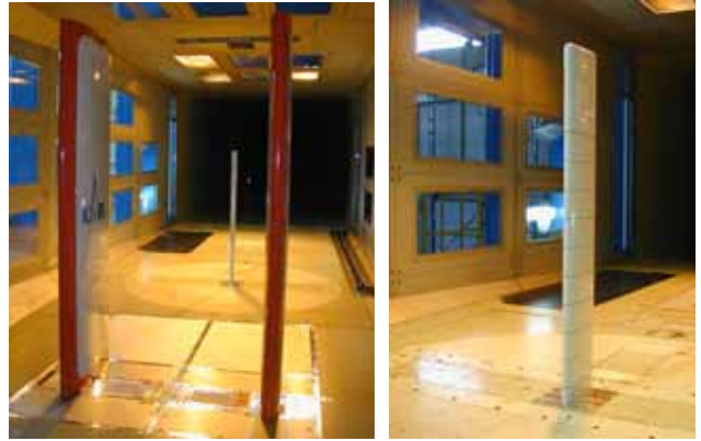
Fig. 5 Gust Response Measurement Wind Tunnel Test for Flexible Wing
