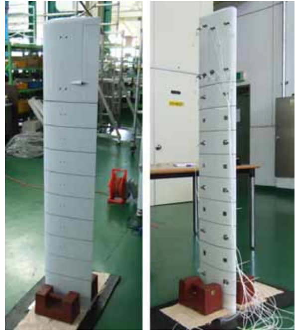
Fig. 2 Set-up for Flexible Wing Modal Test
