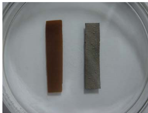
Fig. 1 The strips of the PSMA n -incorporated PVDF before (left) and after (right) Pt electroless-plating. 3 primary reductions and 1 secondary reduction were applied during the fabrication of the INM actuator.
