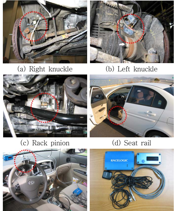
(a) Right knuckle (b) Left knuckle (c) Rack pinion (d) Seat rail (e) Steering wheel (f) Velocity meter Fig. 4 Test tires
