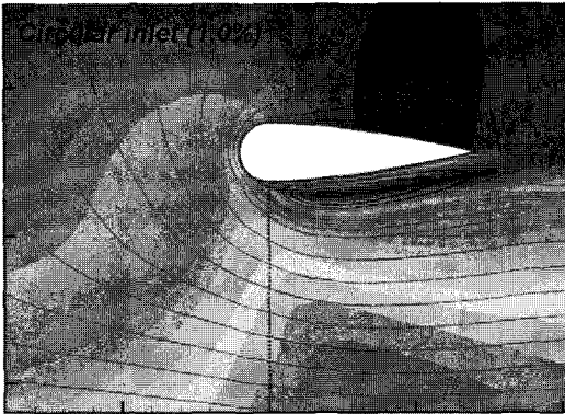
Fig. 8 Flow around duct with circular inlet (gap=1.0%R)
