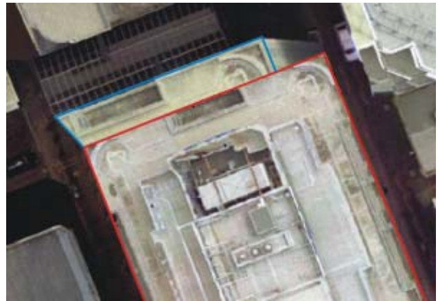
Figure 1. The ghost image of the roof is outlined in blue, the ortho-rectified location in red.
