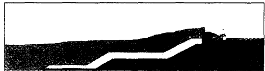
Fig. 2. Snapshot of overtopping(Type-B).
