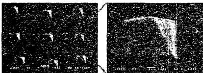
Fig. 3 Micro pyramids on the nickel stamper
