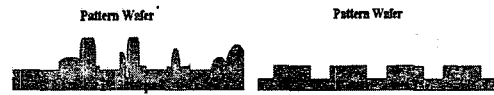
(a) General pad (IC1400-k) (b) MS pad Fig. 3 schematic of contact between pad and pattern wafer
