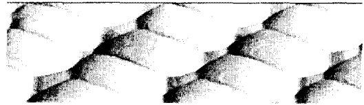
Fig. 13 Unfolded smoked foil record of four walls for the 3-D spinning detonation; detonation propagates left to right.
