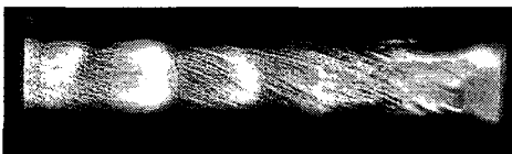
Fig. 9 Typical photograph of PMMA solid fuel during combustion period (oxygen mass flow rate = 0.045kg/s)
