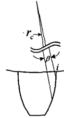
Fig. 7 An involute gear tooth
