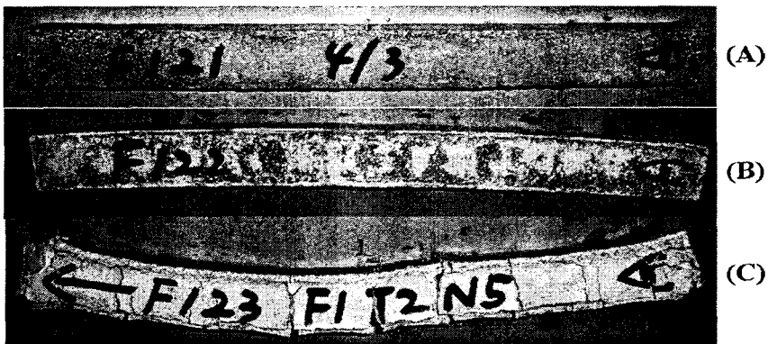
Fig. 3. Mortar specimens with alkali-free accelerator, (A) 2.5% Na 2 SO 4 , aq., (B) 5% Na 2 SO 4 , aq., (C) 10% Na 2 SO 4 , aq.
