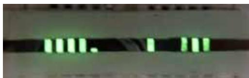
Fig. 9 OLEDs fabricated from Alq 3
