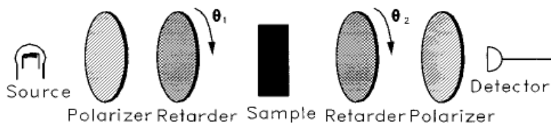
Fig. 1 Schematic diagram of Dual Rotating Retarder Polarimeter
