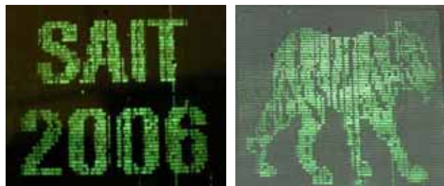
Figure 5. A still cut of moving image displayed on an AMOLED.
