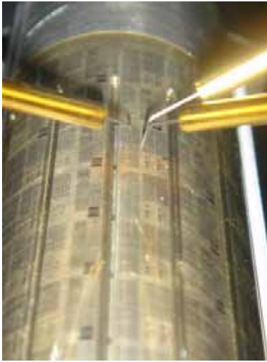
Fig. 2. The a-Si:H TFTs backplane are bonding on camber chuck and vacuumed to fix for electrical measurement. There are three camber chucks with curvature radius 10 cm, 5 cm, and 2.5 cm were used to apply the mechanical strain.
