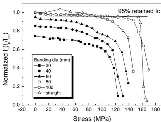
**Fig. 2. Tension stress dependence of critical current for Bi-2223/Ag tapes deformed with various bending diameter.**
