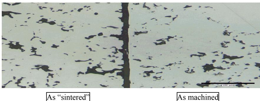
Fig. 10. Samples compacted to the density 7.0 g/cm<sup>3</sup> (left) and 7.5 g/cm<sup>3</sup> (right). Section across the “as sintered” surface with open porosity and “as machined” surface with thin densified layer and closed porosity. Not etched. X100
