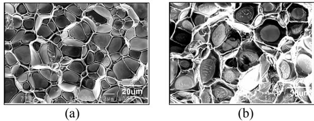
**Fig. 3. Scanning electron micrographs of fracture surface of hybrid structure WHA. (a) Core - Brittle fracture and (b) Housing - Ductile fracture.**
