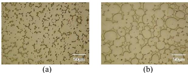
**Fig. 2. Final microstructure of core and housing materials. (a) Core and (b) Housing.**
