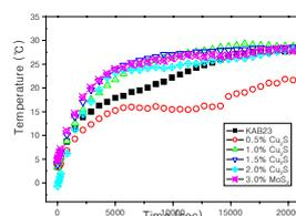
**Fig. 3. Changed of sintered materials during the bearing test for 1 hour powders.**
