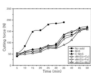
**Fig. 1. Effect of 0.5 wt% MnS and xMnS MnS and xMnS (x = 6wt%) additions on cutting force with machining time increasing.**
