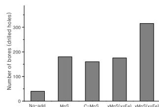
**Fig. 2. Effect of 0.5 wt% MnS and xMnS (x = 6wt%) additions on tool life**
