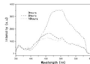
**Fig. 4. Luminescence spectra of mechanically alloyed ZnS for various times.**
