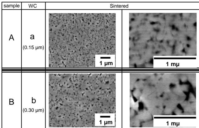
**Fig. 2. Scanning electron microscope images of cemented carbides made from the WC powders of 0.15  $\mu\text{m}$  and 0.3  $\mu\text{m}$  grade.**
