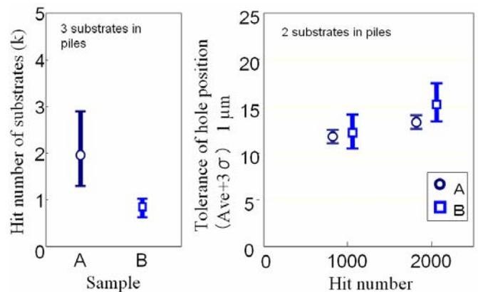
**Fig. 3. Drilling performance of sample A and B (rotational speed: 250kmin<sup>-1</sup>, feed :5  $\mu\text{m}$  /rev and substrate: CCL-HL832HS).**
