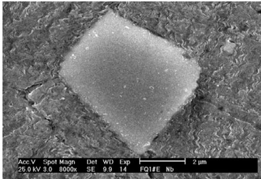
Fig. 1. A NbC particle embedded in matrix.
