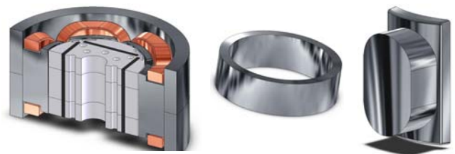
Fig. 3. Cut view of Somaloy stator (left) with small copper end windings, tooth component (right) and core-back (middle).
