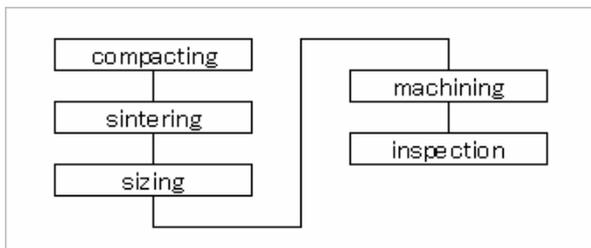
**Fig. 1. Product process of oil-pump**
