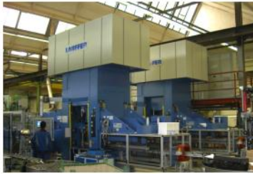
Fig. 2. Multi Function Sizing Centre with two 300 ton presses
