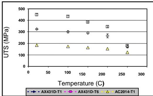
**Fig. 1. Elevated temp.tensile testing for AX 431 Nr .10490 MPa –bars ,as sintered, for both T1 and T6 condition. (4)**
