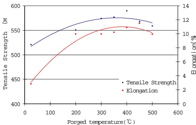
**Fig. 2. Influence of forging temperature on tensile strength and elongation for sinterforged AX 431 Nr.10490**
