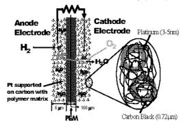
The benchmark is Nafion™ for the membrane and electrodes
