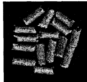
Fig 4. Pellets made by ring die press.
