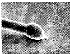
Fig. 5 Result of wire to thin film welding
