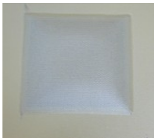
Fig. 3. A forming sandwich of high frictional resistance prepreg
