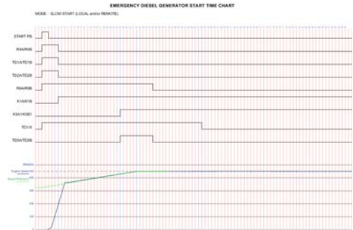
Fig. 3 The sequential timing diagram of diesel engine slow start
