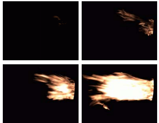
FIG. 14 Ignition flame shape wide burner
