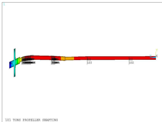
Fig. 2 Analysis of shaft deflection by propeller weight
