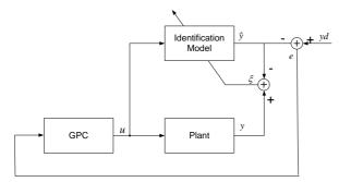
Fig. 2 Block diagram of control system.
