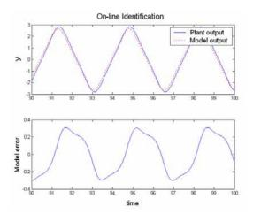
Fig. 4 The on-line ID of The Duffing system.
