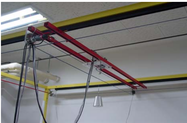
Fig. 3 The 3-D pilot crane used in experiment: InTeCo 3DCrane (Poland).
