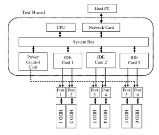
Fig. 3. Architecture of a Test Board
