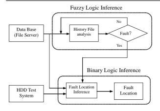
Fig 5. Overall structure of the Expert System
