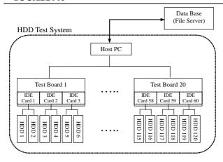
Fig. 2. Architecture of a HDD Test System
