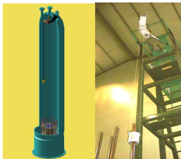
Fig. 1. Pressurizer and robot system in a real size mock-up.
