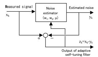
Figure 9. Block diagram of the adaptive self-tuning filter
