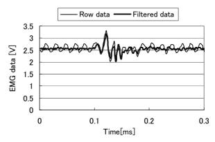
Figure 10. Experimental result of the adaptive self-tuning filter
