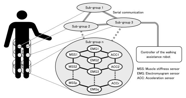
Figure 3. Overview of the sensor network system
