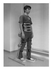
Figure 1. The walking assistance robot
