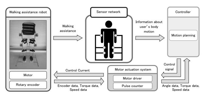
Figure 2. Control system of the walking assistance robot
