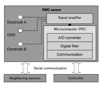
Figure 6. Configuration of the EMG sensor
