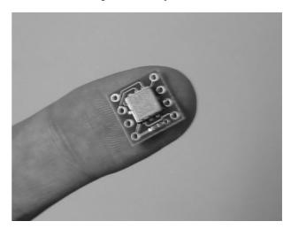
Figure 7. Accelerometer (ADXL202, Analog Devices, Inc)
