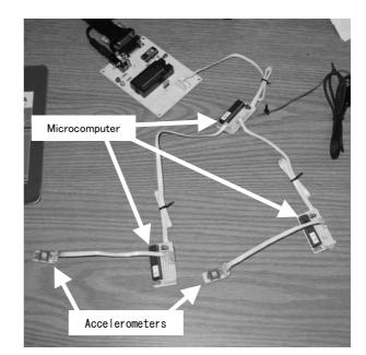
Figure 11. Prototyped network of acceleration sensor
