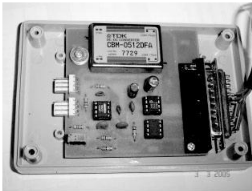
Fig. 11 Amplifier of strain gauge output signal
