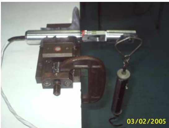
Fig. 13 Designed wrench in weighing system
