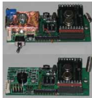
Fig. 3 Receiver (upper) and RF beacon (lower) modules
