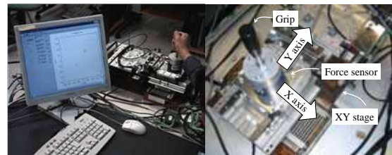
Fig.4 HAM test system with haptic device
