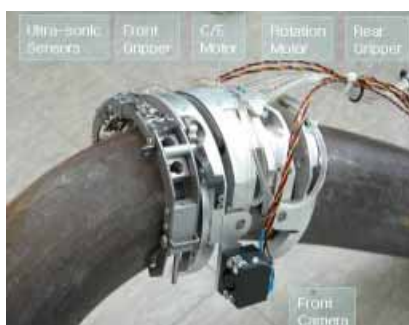
Fig. 4 Feeder pipe inspection robot.
