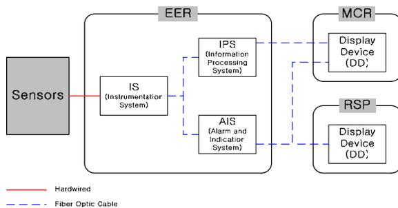
Figure 2. Monitoring interface between MCR and RSP
