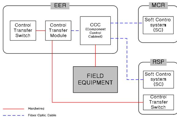
Figure 1. Control interface between MCR and RSP
