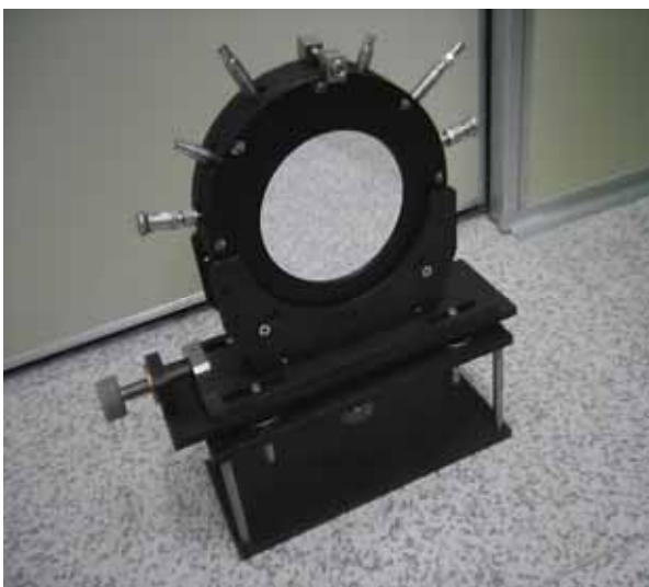
Fig.1 Fabricated parallel plate ionization chamber had double BNC connectors, SHV connectors and gas quick connectors.
