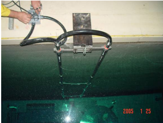
Figure 3. The NDA detector assembly used for the measurement of the basket during the loading (D1).
