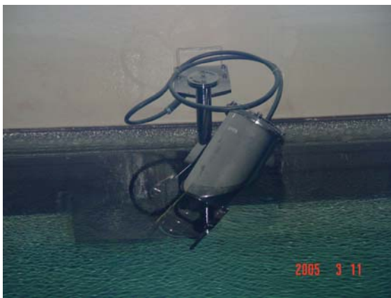
Figure 4. The underwater camera system used for the counting of the basket during the loading (C1 and C2).
