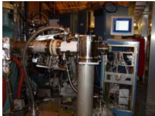
Figure 1. Experimental layout of the proto-type of the X-ray imaging crystal spectrometer installed on Alcator C-MOD tokamak at MIT.
