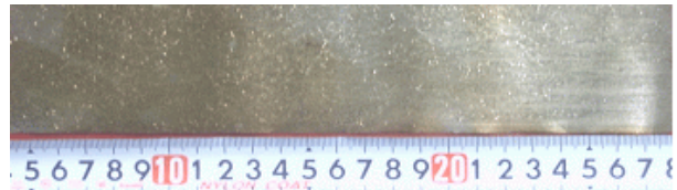
Fig. 1. U-7wt.%Mo foil fabricated by a single roll casting method.
